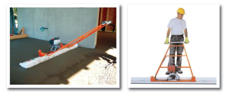
**HERON** is a versatile newly designed vibrating power screed board, created for levelling, compacting and finishing semi-dry floor screed, in preparation for subsequent floor laying. It can also be used to level coarse and fine aggregates. It is equipped with a component which converts motor energy into horizontal orbital movement, producing micro-vibrations of variable intensity, based on the density of the screed.
